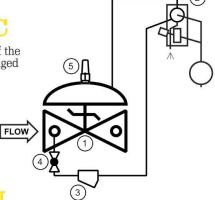
The Model A8000 is designed for tank fill only. A rotary, 3-port, float activated pilot controls the main valve. With the float at the low position on the rod, the pilot shifts to vent water from the diaphragm chamber of the main valve. This allows the valve to open and fill the tank. When the float/fluid level reaches the high position, the pilot shifts to apply full valve inlet pressure to the diaphragm of the main valve, forcing the valve fully closed.
