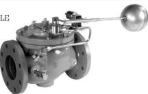
While most Model A8000 Float Valves are line size, there are two factors to check. To keep from using too small a valve, flow rate should be limited to a maximum velocity of 25 ft/sec. Too large a valve can result in loss of inlet pressure, which is needed to close the valve on high level. Consult the factory for assistance.
